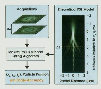
Model-fitting of the diffraction rings in planes through the point spread function (PSF) leads to the precise localization of particles. Courtesy of François Aguet.
